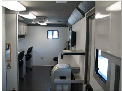
Two axle, 24 'trailer, roof platform, awning, 10KW generator & fuel tank, shore power, galley, restroom with electric toilet, (4) workstaions, (2) A/C, (4) Kwil Raze lights, (1) 15" LCD, (1) 20" LCD, DVD/VCR, (6) scene lights, paging system, (1) equipment rack,(1) restraint chair & hot/cold electric water cooler
